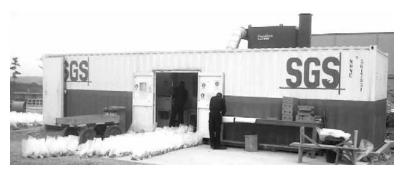
SGS offers sample preparation services globally and has many Mobile Sample Preparation Units (MSPU) in some of the most remote locations in the world. Our MSPUs allow you to access our trusted third party sample preparation services in locations that might not otherwise be supported by laboratory facilities. An SGS-designed, staffed and operated MSPU provides
