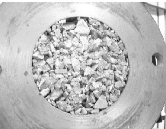
Figure 13: Unbroken rock seen at the bottom of the 100mm diameter cylinder after testing
