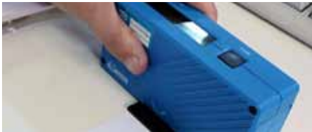
Fig.6: Measurements of gloss or specular reflection according to standard NFT30-064 (ISO2813)
