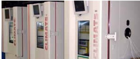
Fig. 7: Over 100 hot/cold/humid climatic chambers with capacities of up to 30 m3
