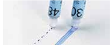
Fig. 9: Application of the test solution to the test surface
